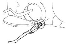
The operation of the sidestand should be checked before each ride, and the sidestand pivot and metal-to-metal contact surfaces should be lubricated if necessary.
