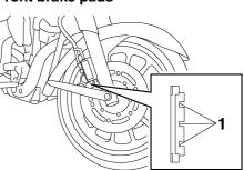
1. Brake pad wear indicator groove
