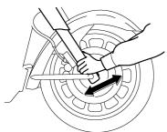
Checking the wheel bearings
