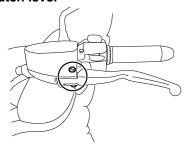
The operation of the brake and clutch levers should be checked before each ride, and the lever pivots should be lubricated if necessary.
