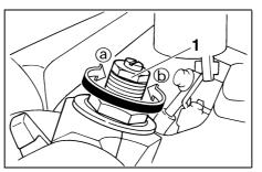
1. Spring preload adjusting bolt
