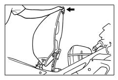
4. Tilt the front of the fuel tank back to position the tank away from the air filter case, and then support the tank as shown.
