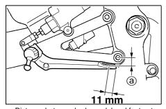
a. Distance between brake pedal and footrest bracket
