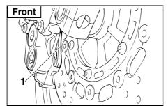
1. Brake pad wear indicator groove
