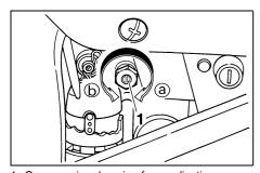
1. Compression damping force adjusting screw
