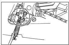
Recommended lubricant: Lithium-soap-based grease (all-purpose grease)
