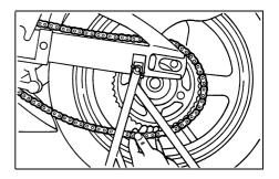
Push the wheel forward, and then remove the drive chain from the rear sprocket.
