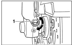
1. Compression damping force adjusting screw
